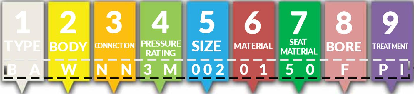
EXAMPLE BA1NN3M0020150FPH BALL VALVE ONE PIECES NPT X NPT CLASS 3000 PSI 1/8" A105N FULL BORE PHOSPHATED
