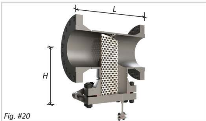
Tee type strainers (straight Flow – W screen) - RF / BW
